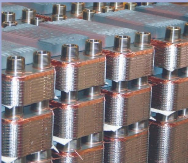
The plate pack, assembled with two end plates and connections, is vacuum brazed at extremely high temperatures providing a permanently sealed heat exchanger. The final result is a strong and compact plate heat exchanger with extremely high heat transmissions. The high heat transmission comes from the main pattern which is designed to create a turbulence flow.
